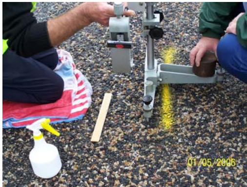
Figure 5. British Pendulum test on a 70/30 blend
