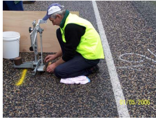
Figure 6. British Pendulum test on a 85/15 blend
