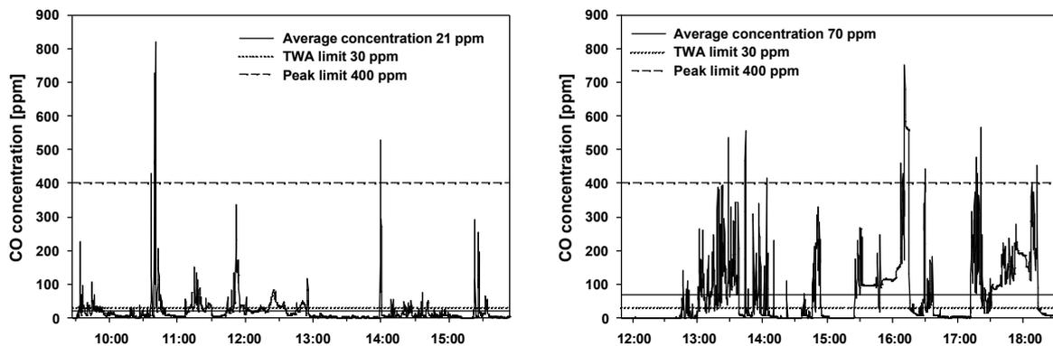
**Figure 2** Data-logging records of firefighter's exposure to carbon monoxide
